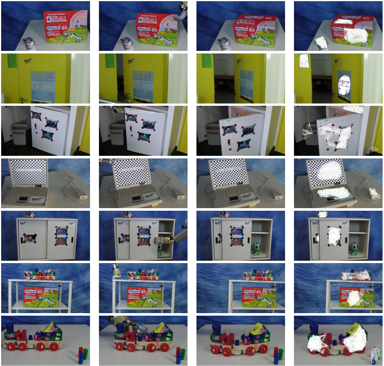
Fig. 9. Experimental results showing the process of identifying rigid bodies in a scene using interactive segmentation. Left to Right: The first column shows the object before the interaction; the second column shows the interaction itself; the third column shows the object after the interaction; and the fourth column shows the results of segmenting the graph of tracked features into clusters of features on the same rigid body.
