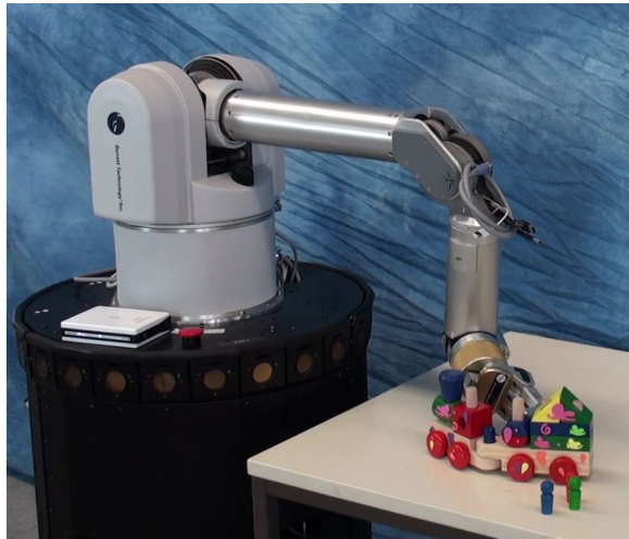
Fig. 1. Our Mobile Manipulator interacts with a train toy, and identifies a set of rigid bodies: train engine, train car, and wooden figures. These rigid bodies are segmented from the background throughout the interaction.
